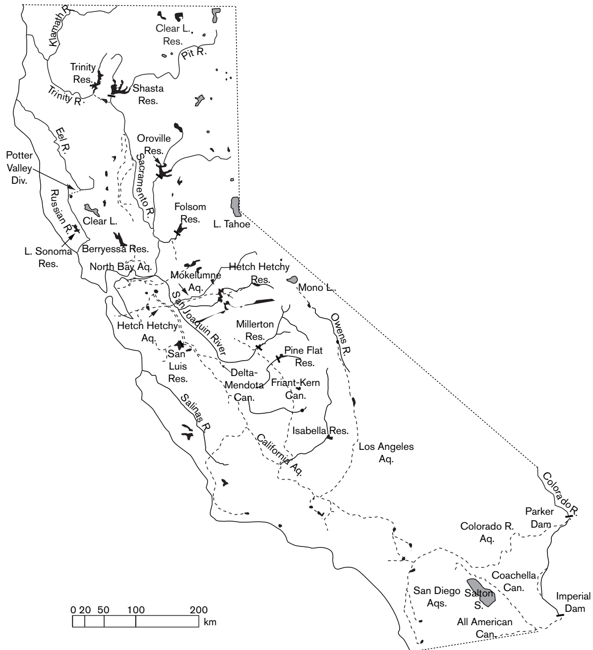
FIGURE 33.7 Major components of the California water storage and delivery system. Major rivers are shown with solid lines, aqueducts and canals as dashed lines, dams as bars, reservoirs as black bodies without outlines, and lakes as gray bodies outlined in black. Map by Parker Welch, Center for Integrated Spatial Research (CISR).
