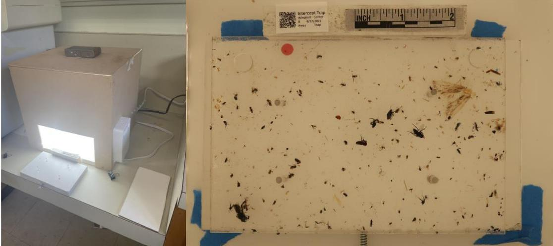
**Figure 7.** Example of light box (left) used for photographing insect sticky traps. The sticky traps are placed on the pegs next to the scale bar and label, and then moved into the box to be photographed (right). Dots, such as the one in the photo on the right, are placed on the side that faces the light for future orientation.
