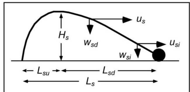
**Figure 3.** Saltation trajectory definition sketch. Shown are the saltation hop height ( $H_s$ ), mean downstream sediment velocity ( $u_s$ ), mean vertical descent velocity ( $w_{sd}$ ), horizontal ( $u_{si}$ ) and vertical ( $w_{si}$ ) impact velocities, and the upward ( $L_{su}$ ) and downward ( $L_{sd}$ ) portions of the total hop length ( $L_s$ ).
