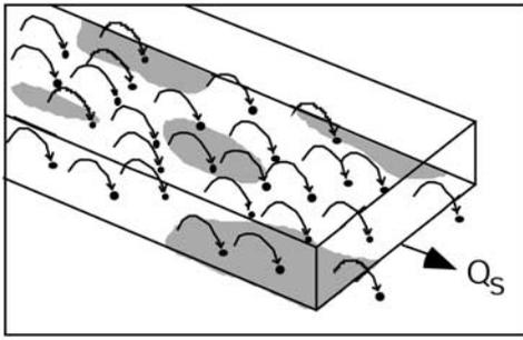
**Figure 2.** Idealized rectangular channel eroded by saltating bed load impacts. Shaded areas represent transient alluvial deposits that shield underlying bedrock from erosive effect of bed load sediment flux ( $Q_s$ ).
